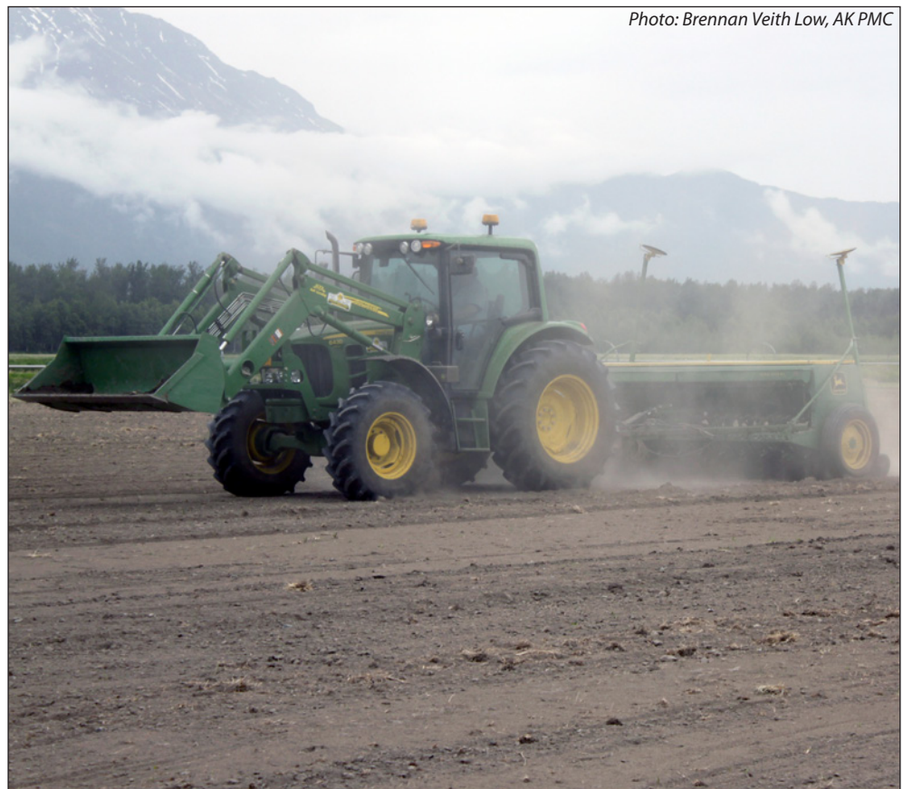
A drill seeder is towed behind a tractor at the Alaska PMC
